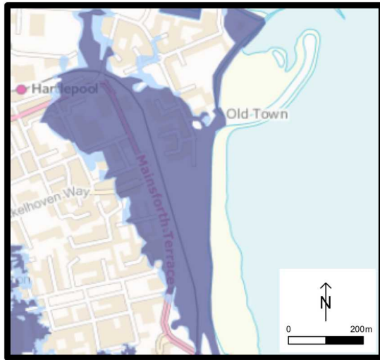
Figure 2. The benefit area – the likely flood extent in the northern UK town of Hartlepool. The dark shade is the 100-year return period outline; the lighter shade the 1,000 year return period.
